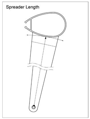
(ii) HEIGHT: The distance between **mast datum point** and the intersection of the lower edge of the **spreader**, extended as necessary, and the **mast spar**.
